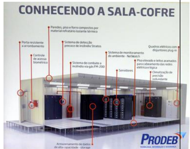
Layout of PRODEB data center safe room
